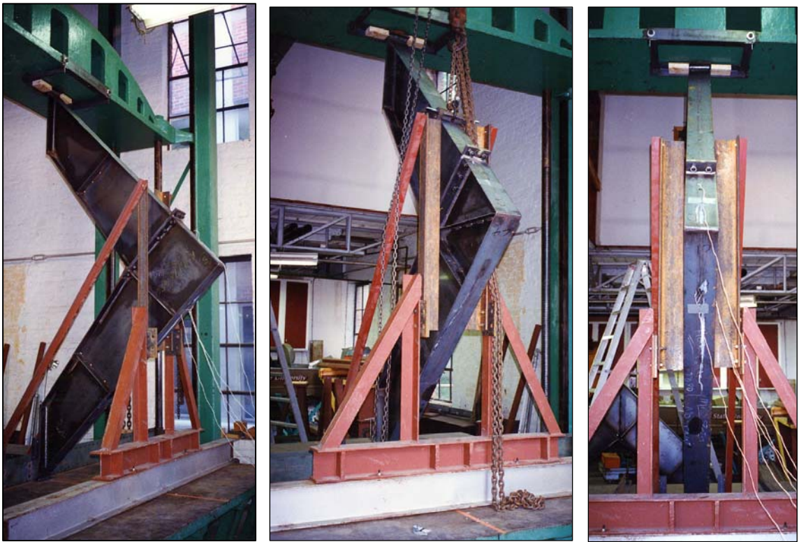
Figures 2.6, 2.7 and 2.8 Test setup for all five frames with lateral guide angles
