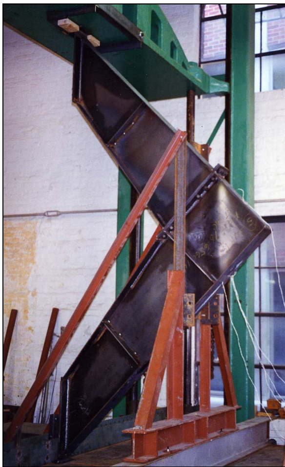
Figure 4.6 Buckling in knee web of frame 1 (frame 3 was identical)
